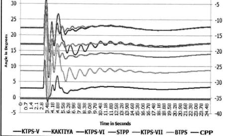
Internal cable/Line fault at CPP isolated
